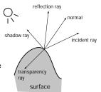
Shadow rays stop at light sources, but reflection and transparency rays behave just like primary rays!
