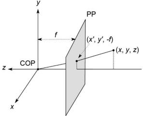
The distance f is called the **focal length** of the pinhole camera , as it is essentially equivalent to the focal length of a lens system in a camera.
