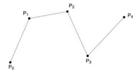
We can specify the Bezier control points directly, or we can devise a scheme for placing them automatically...
