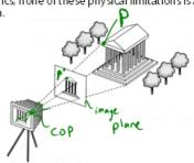
The image is rendered onto an image plane (usually in front of the camera).
