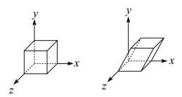
We call this a shear with respect to the x-z plane.
