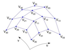
Given a grid of control points  $V_{ij}$ , forming a **control net**, contruct a surface S(u,v) by:
