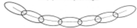
FIGURE 4c. Stretching the object so that its positions overlap again will relieve the strobbling effect.
