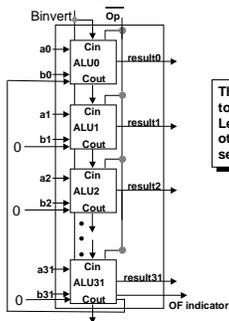
The Set line feeds back to become the input to Less for bit-0. All other bits have Less set to zero.
