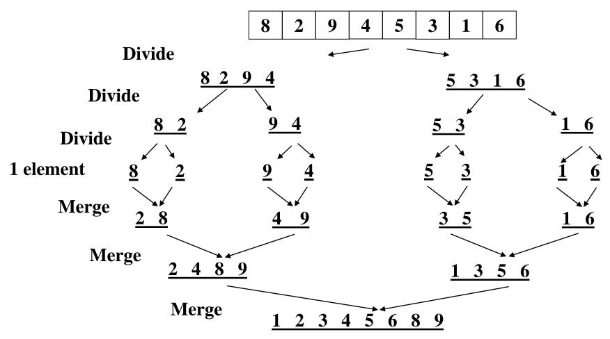
We need another array in which to do each merging step; merge results into there, then copy back to original array 36
