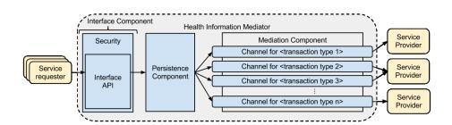
Fig. 2. Overview of components in the HIM architecture
