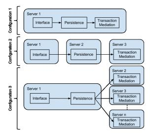
Fig. 4. Scalability configurations of the HIM architecture
