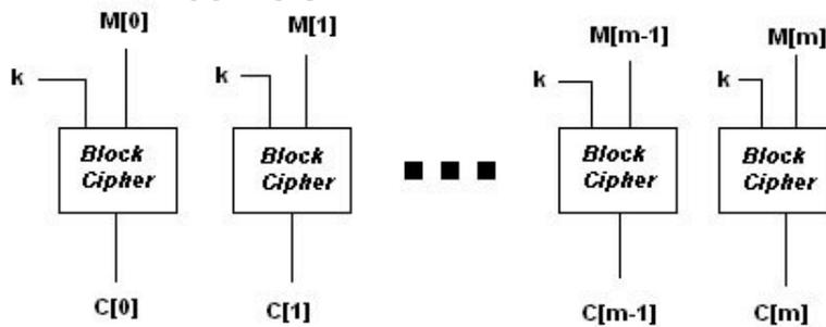
Figure 1 – Electronic Code Book (ECB) mode encryption algorithm
