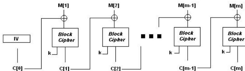
Figure 2 - CBC Encryption Algorithm
