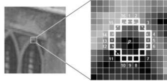
Figure 1. 12 point segment test corner detection in an image patch. The highlighted squares are the pixels used in the corner detection. The pixel at  $p$  is the centre of a candidate corner. The arc is indicated by the dashed line passes through 12 contiguous pixels which are brighter than  $p$  by more than the threshold.
