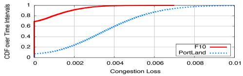
PortLand has 7.6x the congestion loss of F10 under realistic traffic and failure conditions
