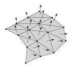
For surfaces of revolution, we can get better-looking results by analytically computing the normal at each vertex...
