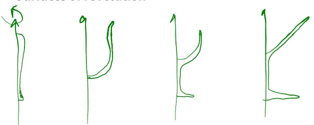
Idea: rotate a 2D **profile curve** around an axis.
