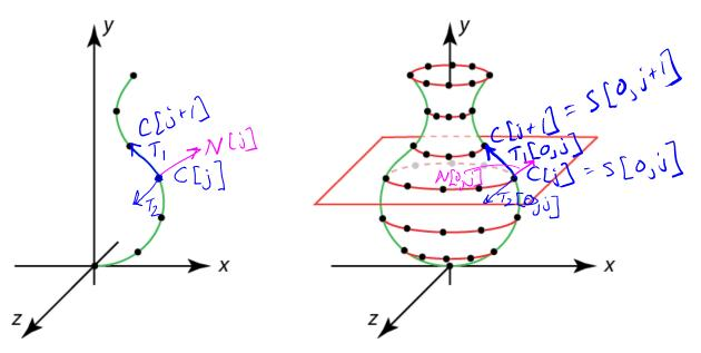
We can compute tangents to the curve points in the x-y plane:
