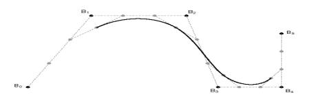
These are called  ${\bf B}\text{-splines}$ . The starting set of points are called  ${\bf de}$   ${\bf Boor}$   ${\bf points}$ .
