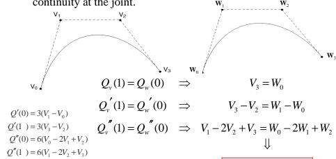
$$W_2 = V_1 + 4V_3 - 4V_2$$
