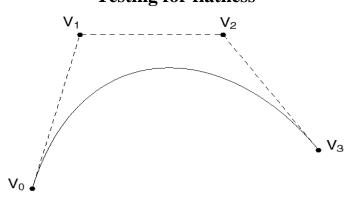
Compare total length of control polygon to length of line connecting endpoints:
