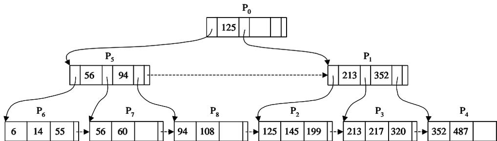
**Figure 6.18** The B-Tree of Figure 6.17 After Inserting 60 Page P<sub>7</sub> is split into P<sub>7</sub> and a new page P<sub>8</sub>, links are updated, and the boundary key 94 is inserted in page P<sub>5</sub>.
