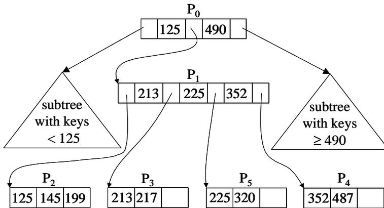
**Figure 6.15 A B-Tree After a Split** This shows the B-tree of Figure 6.18 after inserting key 225, assuming P<sub>1</sub> can hold 3 keys.
