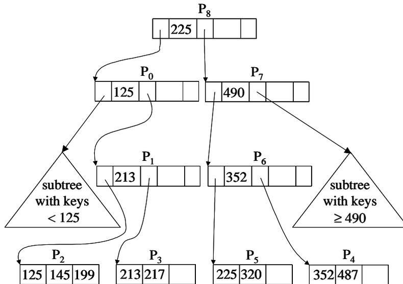
**Figure 6.6 A B-Tree After a Recursive Split** This shows the B-tree of Figure 6.15, after inserting key 225, assuming  $P_1$  can hold at most 2 keys. Thus,  $P_1$  must split into  $P_1$  and  $P_6$ , which in turn causes  $P_0$  to split into  $P_0$  and  $P_7$ , which causes a new root  $P_8$  to be created.
