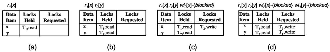
**Figure 6.3 Execution Leading to a Deadlock** Each step of the execution is illustrated by the operations executed so far, with the corresponding state of the lock table below it.
