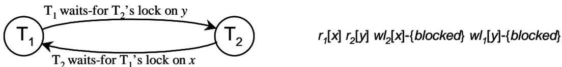
**Figure 6.5 A Waits-For Graph** The graph on the left represents the waiting situations in the execution on the right (see also Figure 6.4). Since there is a cycle involving  $T_1$  and  $T_2$ , they are deadlocked.
