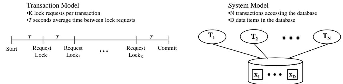
**Figure 6.9 Mathematical Model of Transactions and System.** Using this model, formulas can be derived for probability of conflict and deadlock and for throughput.
