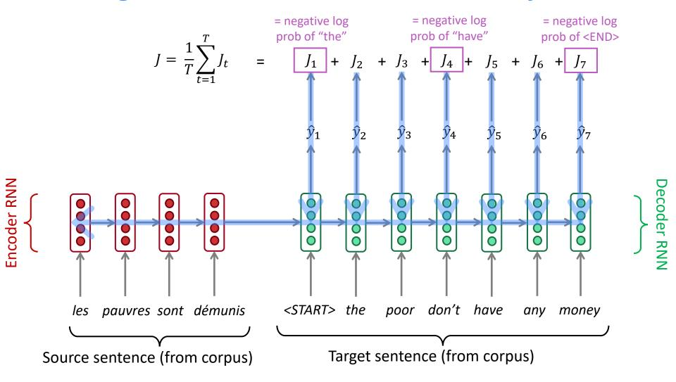
Seq2seq is optimized as a <u>single system.</u> Backpropagation operates "end to end".
