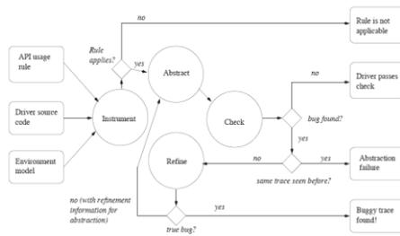
Figure 5: SDV's analysis engine's architecture
