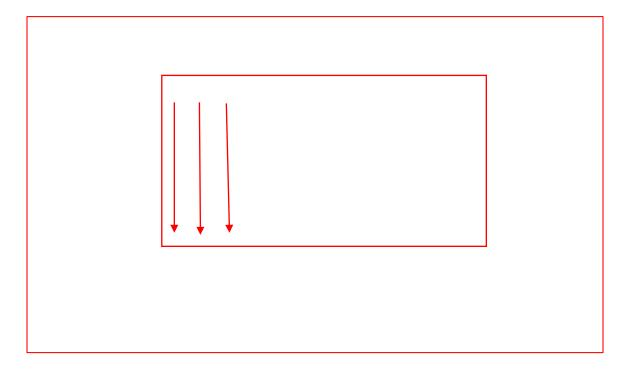
Successive writes to elements of the array will require reading a new cache line. The program does not benefit from caching.
