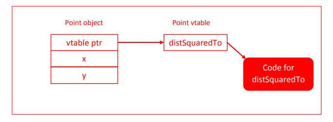
Note that because Point has no implicit base class, the only entry in its vtable is a pointer to the distSquaredTo function (so no entries for inherited virtual methods, such as *hashcode* or *toString*, for example)
