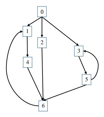
A. 10 points. For each node in the above flowgraph (or control-flow graph), list its Predecessors, Successors; the nodes that it dominates; the nodes that dominate it – by filling in the table below:
