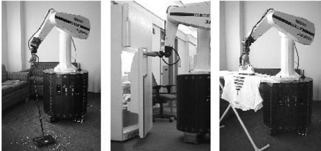
Fig. 12. Experiments with the Stanford Mobile Platforms: vacuuming, opening a door, and ironing are examples of tasks demonstrated with the Stanford Mobile Platforms.
