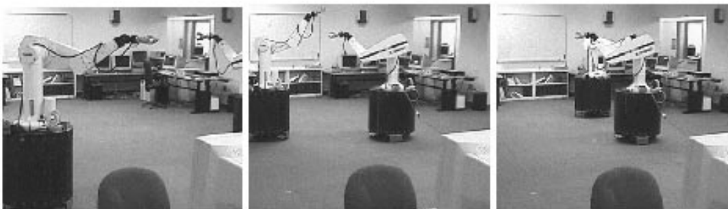
Fig. 11. Experimental Execution of a Plan: the path of the first platform is modified in real-time to avoid the second moving platform.
