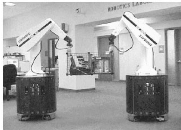
Fig. 1. The Stanford robotics platforms: two holonomic platforms, each is equipped with a PUMA 560 arm, various sensors, two computer systems, a multi-axis controller, and sufficient battery power to allow for autonomous operation.
