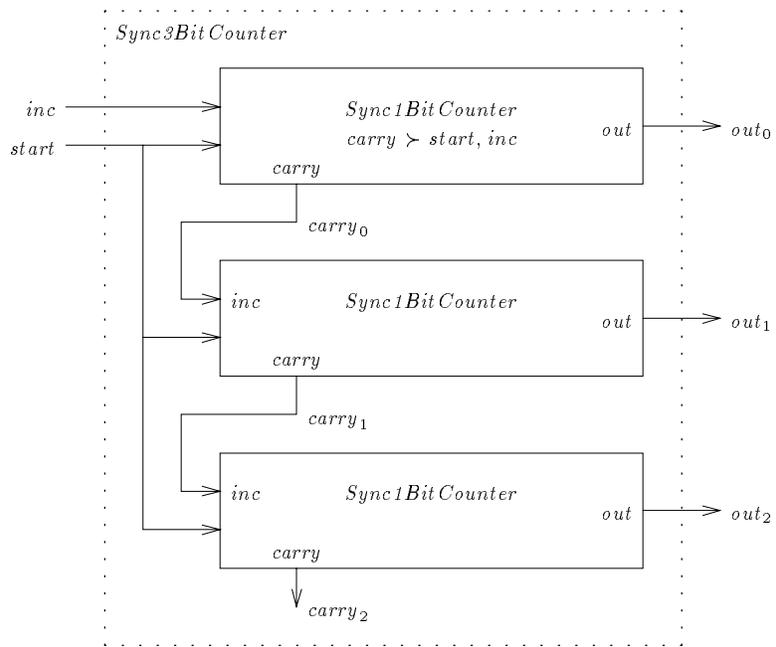
Figure 7: Block diagram for a three-bit binary counter
