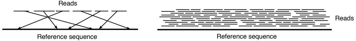
Fig. 1. Reassembly aligns each read to the correct position in the reference sequence. Sufficient redundant reads are generated to cover the reference sequence up to some read depth D .
