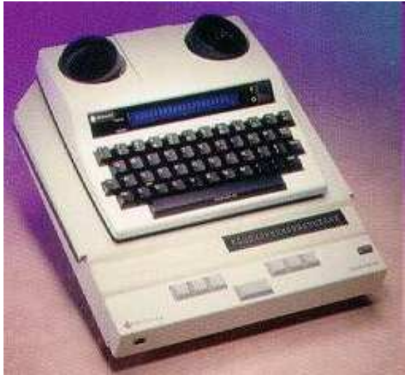
TeleBraille (1984) TTY with Braille output
