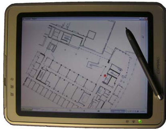
Figure 7: Map GUI running on a tablet PC. Red mark shows participant location and orientation.
