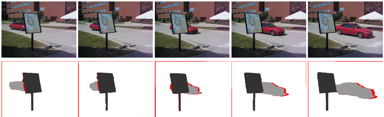
Figure 10: Segmentation results for the car-map sequence. Top: Several frames from the sequence. Bottom: The segmentation results, where the layers are accurately extracted even though the most parts of the moving car are occluded in some frames.
