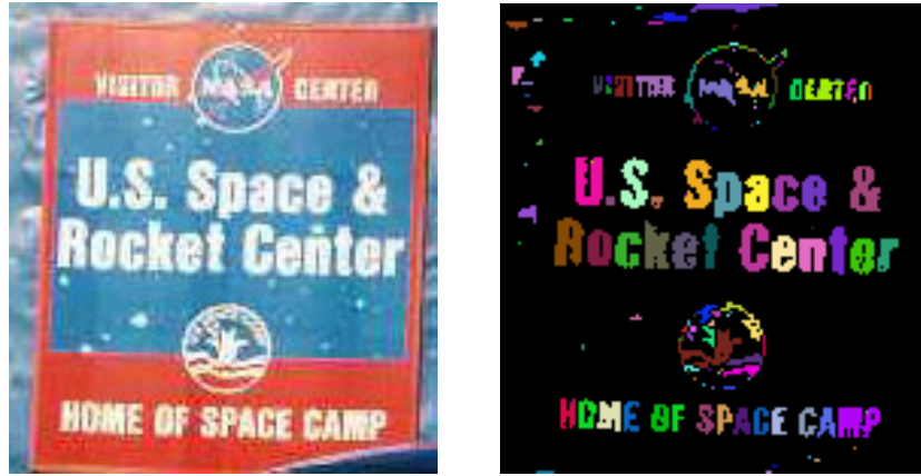
Figure 6.10: “White pixels” are segmented from the color image at the left. Individual connected components of white pixels are arbitrarily labeled by a coloring algorithm as described in Chapter 3. (Analysis contributed by David Moore.)
