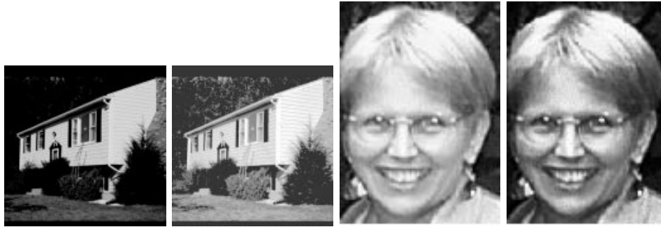
Figure 5.4: Histogram equalization maps the grey scale such that the output image uses the entire range available and such that there are approximately the same number of pixels of each grey value in the output image: images after histogram equalization are at the right.
