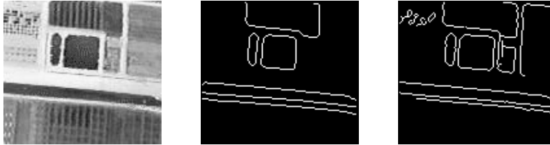
Figure 10.17: Contours from an aerial image of farm fields defined using the Canny operator with \sigma = 2 and \sigma = 1 respectively. Note that five major structures are well represented – three fields and two straight horizontal bands in the bottom of the image (a canal and a road alongside it).
