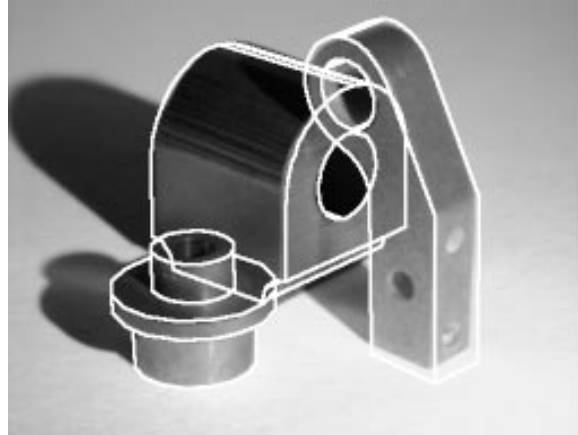
Figure 1.7: An inspection or assembly robot matches stored 3D models to a sensed 2D image (Courtesy of Mauro Costa).
