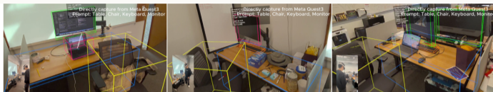
(b) Augmented Reality (Meta Quest 3): passthrough AR with 3D bounding boxes rendered in real time across three different desk scenes.
