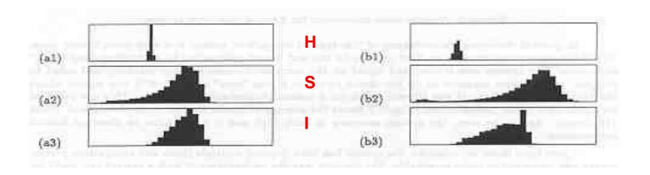
Separate HSI histograms for apples (left) and oranges (right) used by IBM's VeggieVision for recognizing produce at the grocery store checkout station (see Ch 16).
