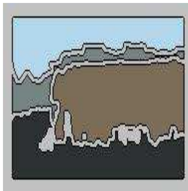
Figure 3: Blobworld EM segmentation of the building scene using color and texture features.
