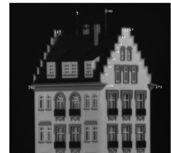
Figure 4.7: For a quantitative evaluation, distances between the features shown in the picture were measured on the actual model, and compared with the computed results. The comparison is shown in figure 4.8.
