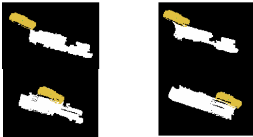
Fig. 5. Object matching process for two occluded vehicles.
