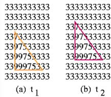
Example of image flow: a brighter triangle moves 1 pixel upward from time  $t_1$  to time  $t_2$ . Background intensity is 3 while object intensity is 9.
