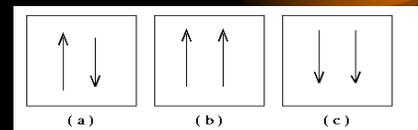
(a) Opposite flow vectors means RUN; speed determined by vector magnitude.
