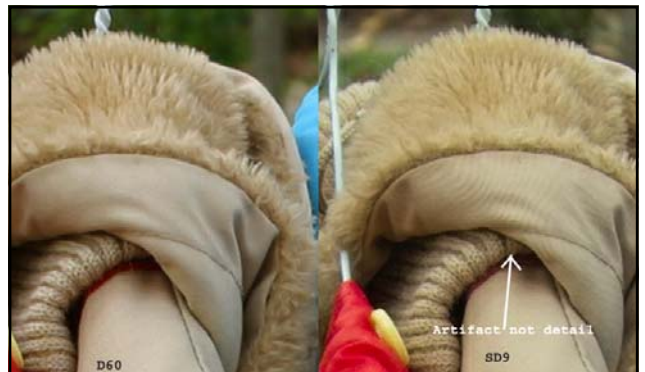
Moiré patterns in real-world images. Here are comparison images by Dave Etchells of Imaging Resource using the Canon D60 (with an anti-alias filter) and the Sigma SD-9 (which has no anti-alias filter). The bands below the fur in the image at right are the kinds of artifacts that appear in images when no anti-alias filter is used. Sigma chose to eliminate the filter to get more sharpness, but the resulting apparent detail may or may not reflect features in the image.
