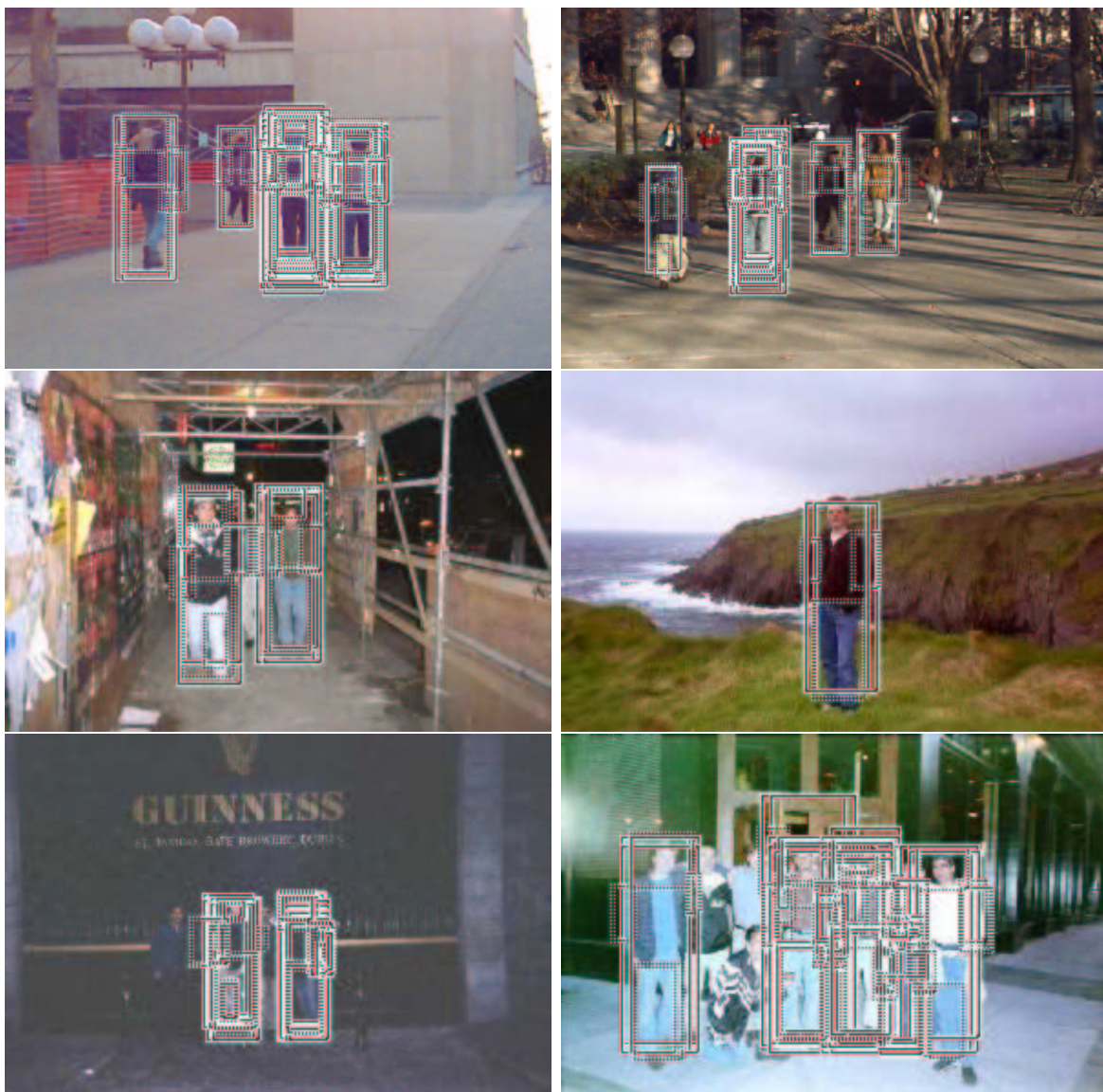
Figure 10: Results from the component based person detection system. The solid boxes outline the complete pedestrian, where the dashed rectangles are the components.
