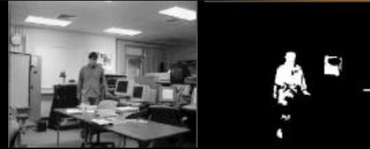
Pixel changes detected as difference regions (components). Regions are (1) person, (2) opened door, and (3) computer monitor. System can know about the door and monitor. Only the person region is “unexpected”.
