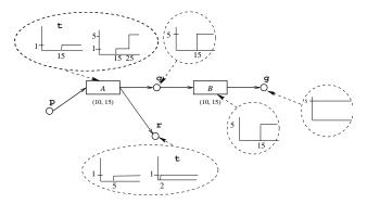
Figure 5: Utility table propagation for conjunctive effects
