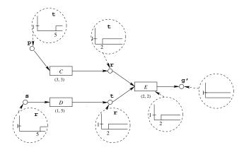
Figure 4: Utility table propagation for conjunctive preconditions
