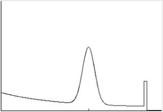
$$P(z|x, m) = \begin{pmatrix} \alpha_{hit} \\ \alpha_{unexp} \\ \alpha_{max} \\ \alpha_{rand} \end{pmatrix}^T \cdot \begin{pmatrix} P_{hit}(z|x, m) \\ P_{unexp}(z|x, m) \\ P_{max}(z|x, m) \\ P_{rand}(z|x, m) \end{pmatrix}$$
