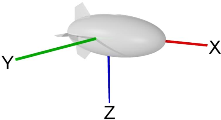
$$\dot{s} = \frac{d}{dt} \begin{bmatrix} p \\ \xi \\ v \\ \omega \end{bmatrix} = \begin{bmatrix} R_b^e v \\ H(\xi) \\ M^{-1}(\sum Forces - \omega^* M v) \\ J^{-1}(\sum Torques - \omega^* J \omega) \end{bmatrix}$$
