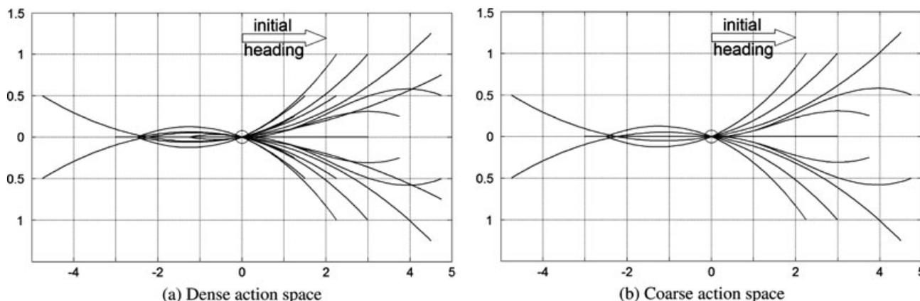
**Figure 12.** Dense and coarse resolution action spaces. The coarse action space contains many fewer actions (24 versus 36 in the dense action space) with transitions only to states with a coarse-resolution heading discretization (in our case, 16 headings versus 32 in the dense-resolution discretization). In both cases the discretization in position is 0.25 m and the axes in both diagrams are in meters.
