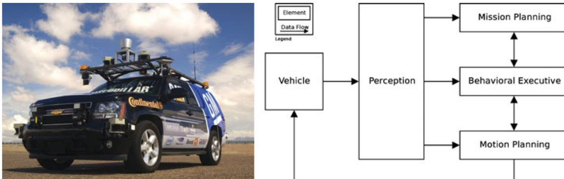
**Figure 1.** Boss: Carnegie Mellon's winning entry in the Urban Challenge, along with its software system architecture.
