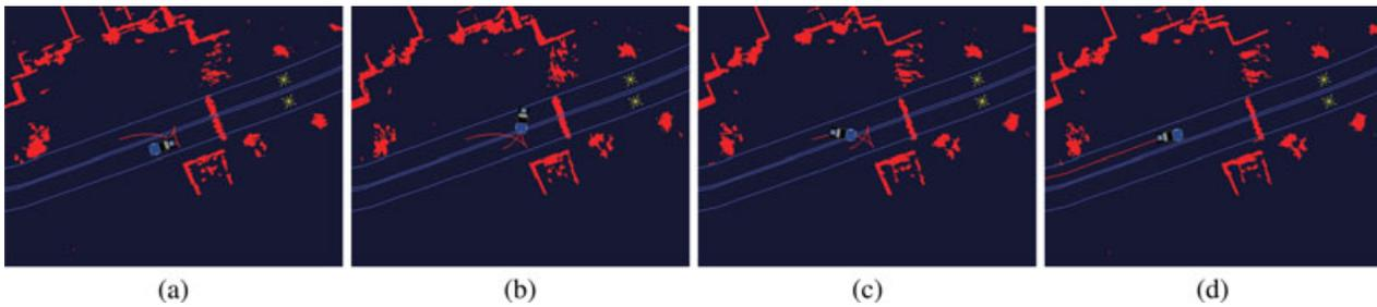
**Figure 9.** Performing a U-turn when encountering a road blockage. In this case the road was too narrow to perform a single forward action to turn around and a three-point turn was required. (a) Initial plan generated to reverse the direction of the vehicle. (b, c) Tracking the plan. (d) Reverting back to lane driving after the vehicle has completely turned around and is in the correct lane.
