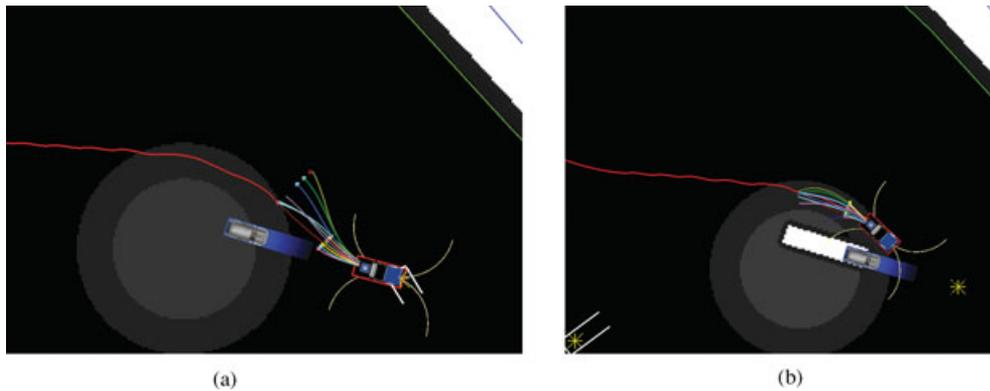
**Figure 17.** Defensive driving when in unstructured environments. (a) Trajectories thrown to right of path (other vehicle should likewise go to right). (b) New path planned from new position.
