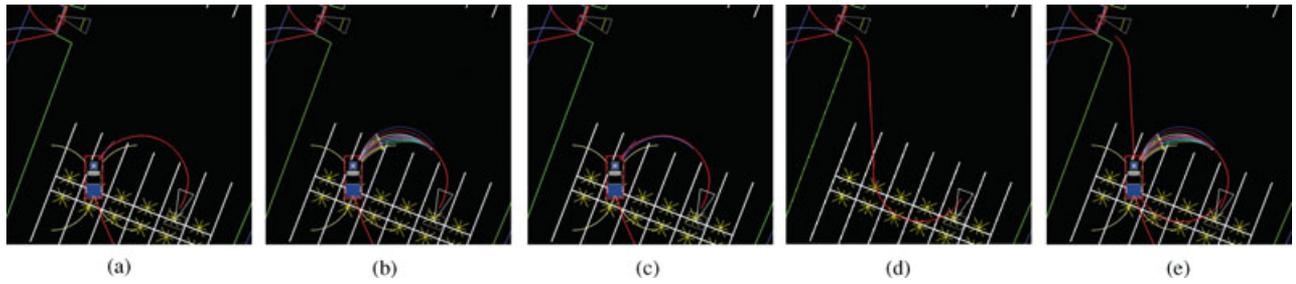
**Figure 15.** Following a lattice plan to a parking spot. Here, one lattice planner is updating the path to the spot while another is simultaneously preplanning a path out of the spot. The goals are represented by the white (current goal) and gray (next goal) triangles.
