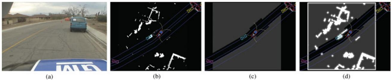
**Figure 13.** Snapshot from a qualification run during the Urban Challenge, showing (b) the obstacle map from perception (obstacles in white), (c) the constrained cost map based on the road structure (lighter areas are more costly), and (d) the resulting combined cost map used by the planner.
