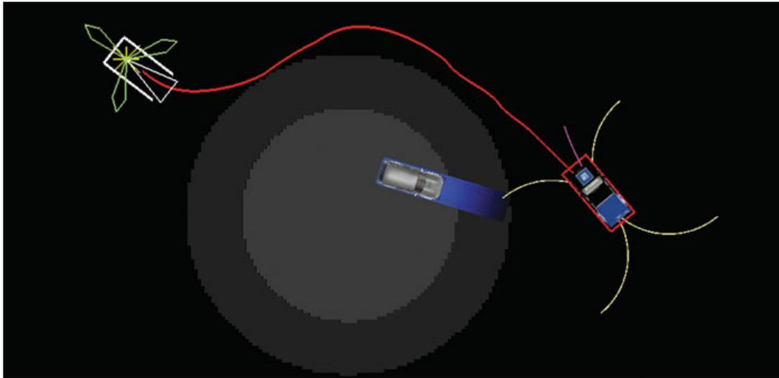
**Figure 14.** Biasing the cost map for the lattice planner so that the vehicle keeps away from dynamic obstacles. Notice that the high-cost region around the dynamic obstacle is offset to the left so that Boss will prefer moving to the right of the vehicle.
