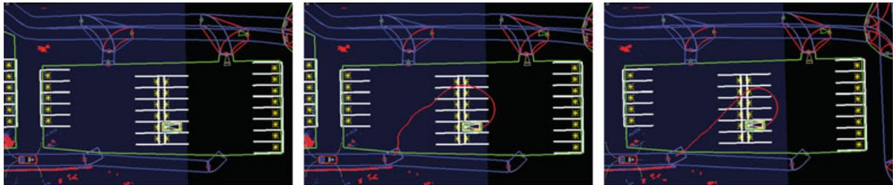
**Figure 19.** Preplanning a path into a parking spot and improving this path in an anytime fashion. A set of goal poses are generated that satisfy the parking spot, and an initial path is planned while the vehicle is still outside the parking lot. This path is improved as the vehicle approaches, converging to the optimal solution shown in the right-hand image.
