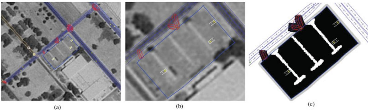
**Figure 18.** Generating constrained cost maps offline for Castle Commerce Center, California. (a) Overhead imagery showing testing area with road network overlaid. (b) Parking lot area (boundary in blue) with overhead imagery showing curb islands. (c) Resulting constrained cost map incorporating boundaries, entry and exit lanes, and curb islands (the lighter the color, the higher the cost).
