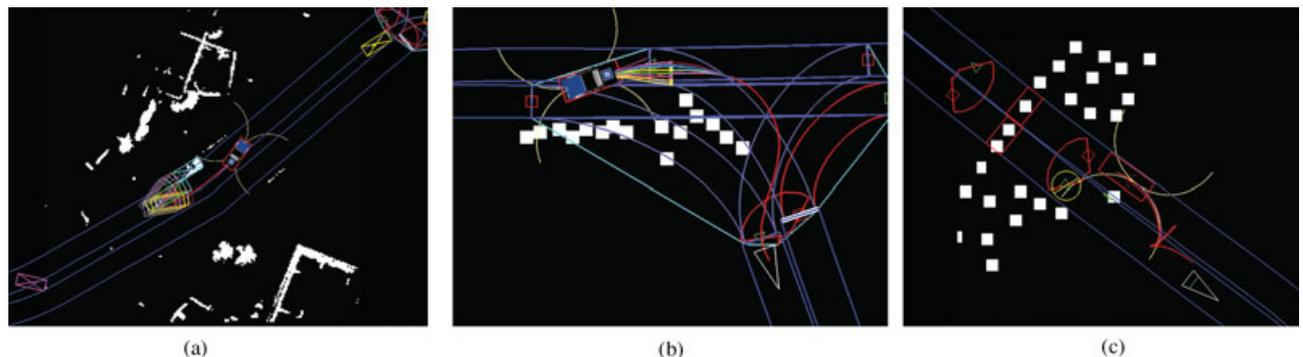
**Figure 20.** Error recovery examples. (a) Planning around a stalled vehicle in the road (obstacles in white, set of pose goals given to planner shown as various colored rectangles, and resulting path shown in red). Corresponds to scenario from Figure 13. (b) Planning through a partially blocked intersection. (c) Performing a complex U-turn in a cluttered area. (Boss's three-dimensional model has been removed to see the lattice plan underneath the vehicle.)
