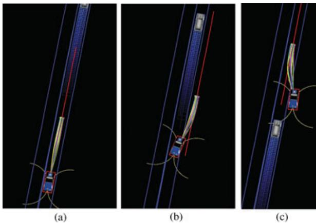
**Figure 10.** Defensive driving on roads. (a) Boss initially plans down its lane while the oncoming vehicle is far away. (b) When the oncoming vehicle is detected as dangerous, Boss generates a set of trajectories off the right side of the road. (c) After the oncoming vehicle has passed, Boss plans back onto the road and continues.
