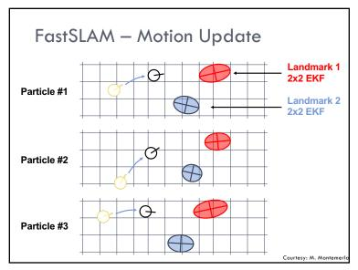
**FastSLAM** □ Proposed by Montemerlo et al. in 2002 □ Each landmark is represented by a 2x2 EKF ☐ Each particle therefore has to maintain M individual **EKFs Particle** |x,y, heta|Landmark 1 Landmark 2 Landmark M Particle  $[x, y, \theta]$ Landmark 1 Landmark 2 Landmark M Particle |x,y, heta|Landmark 2 Landmark 1 Landmark M
