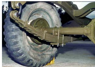
Fig. 1: Leaf spring from http://en.wikipedia.org/wiki/Image:Leafs1.jpg
