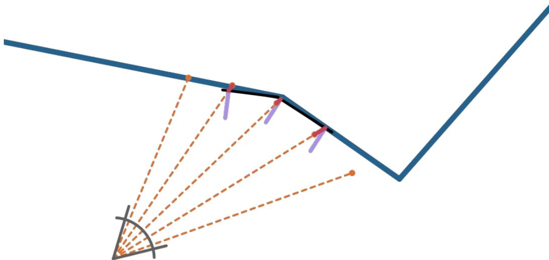
$$\frac{\partial E(\theta \oplus \Delta\theta)}{\partial \Delta\theta} = \sum_i n_i^{\text{pred}} \cdot \frac{\partial}{\partial \Delta\theta} T_{gl}(\theta \oplus \Delta\theta) x_i^{\text{obs}}$$
