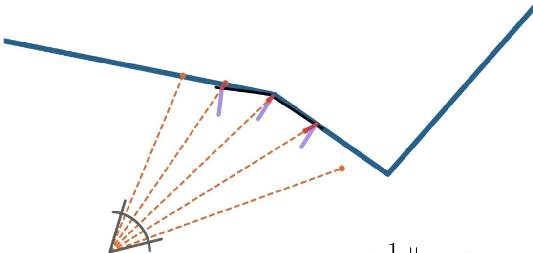
$$E(\theta) = \sum_i \frac{1}{2} \left\| \underline{n_i^{\text{pred}}} \cdot \left( \underline{T_{gl}(\theta)} \underline{x_i^{\text{obs}}} - \underline{x_i^{\text{pred}}} \right) \right\|_2^2$$
