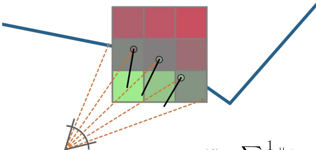
$$E(\theta) = \sum_i \frac{1}{2} \|SDF(T_{gl}(\theta)x_i^{\text{obs}})\|_2^2$$
