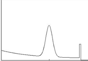
$$P(z | x, m) = \begin{pmatrix} \alpha_{\text{hit}} \\ \alpha_{\text{unexp}} \\ \alpha_{\text{max}} \\ \alpha_{\text{rand}} \end{pmatrix}^T \begin{pmatrix} P_{\text{hit}}(z | x, m) \\ P_{\text{unexp}}(z | x, m) \\ P_{\text{max}}(z | x, m) \\ P_{\text{rand}}(z | x, m) \end{pmatrix}$$
