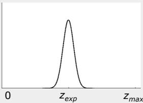
$$P_{hit}(z | x, m) = \eta \frac{1}{\sqrt{2\pi\sigma^2}} e^{-\frac{1}{2} \frac{(z - z_{exp})^2}{\sigma^2}}$$
