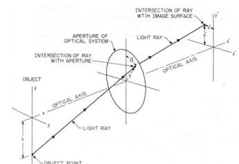
Figure 3.1 A ray from the point  $y = h$ ,  $x = 0$  in the object passes through the optical system aperture at a point defined by its polar coordinates,  $(r, \theta)$ , and intersects the image surface at  $y', z'$ .
