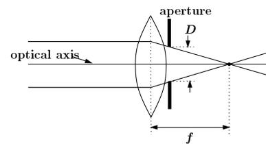
An aperture of diameter,  $D$ , restricts the extent of the bundle of refracted rays.
