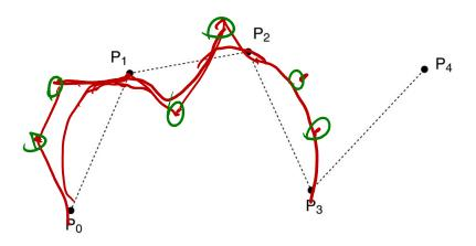
We call this curve a **spline**. The endpoints of the Bezier segments are called **joints**. All other Bezier points (i.e., not endpoints) are called **inner Bezier points**; these points are generally not interpolated.
