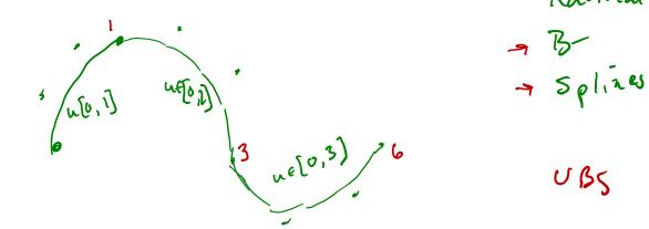
The *u*-range affects placement of control points. The result is a **non-uniform** spline.
