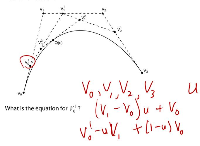
$$V_0^1 = (1-u)V_0 + uV_1$$
