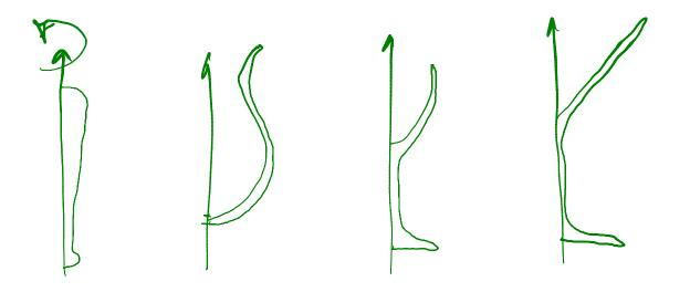
Idea: rotate a 2D **profile curve** around an axis.
